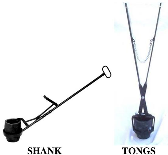
Tongs are used to lift the crucible from the furnace. A shank is used to hold and pour the crucible. Smaller sized crucibles can both be lifted and poured with tongs. You can make your own tongs or buy commercial ones. David Gingery's books show how to make your own. In either case the tongs must fit properly to hold the crucible snugly without crushing it.
